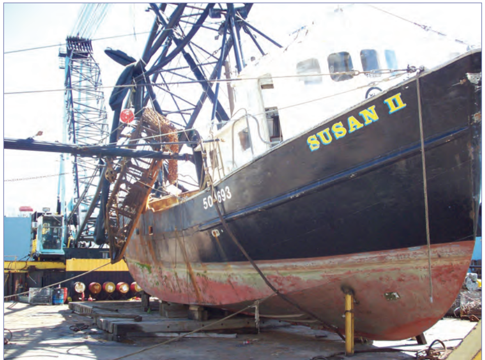
Donjon's 400-ton capacity derrick Columbia New York lifts the Susan II , a clamming boat that sank in Manasquan Inlet.
